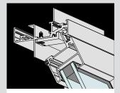
Continuous hinge hood on sashes protects the top of the sash from water intrusion
